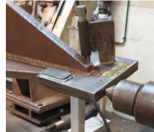
Performance of the center hole inside the plug necessary to set up axial symmetry on machine tool.
